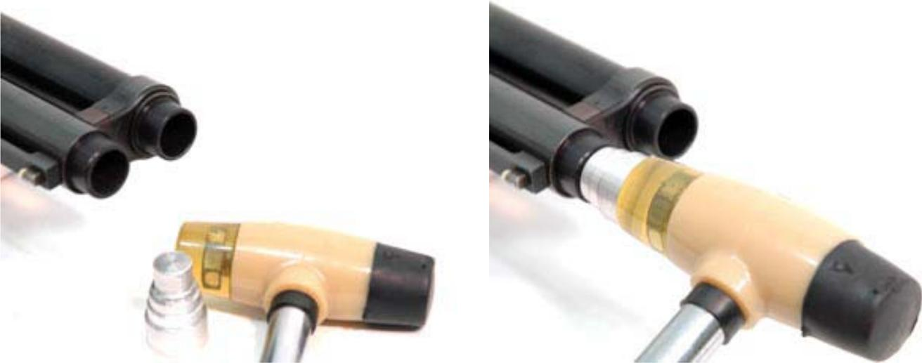
gently tap out the tubes. These tubes are machined to incredibly close tolerances and take very little effort to insert and remove.
