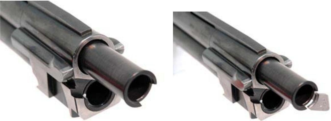
**You can use the ejector to be sure it lines up, then push the tube into the barrel.**
