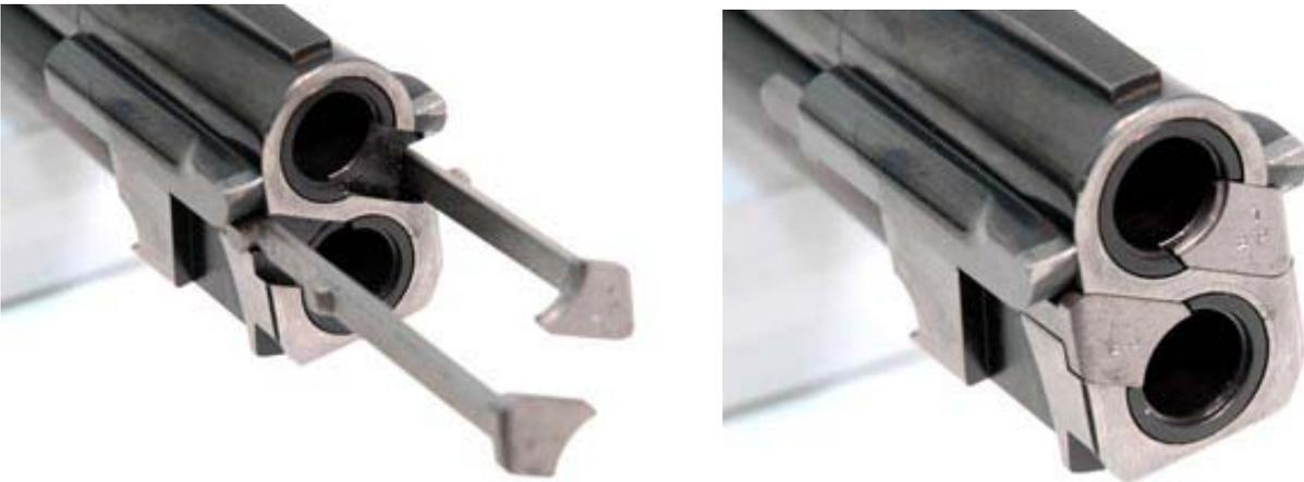
**Finally the ejectors are dropped into place. At this point the ejectors are not restrained**
